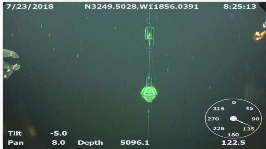
View from the ROV camera showing one of the passive acoustic monitoring buoys in the water column. The ROV claw tool can be shown on the far left and the cutting tool can be shown in the upper right corner.
